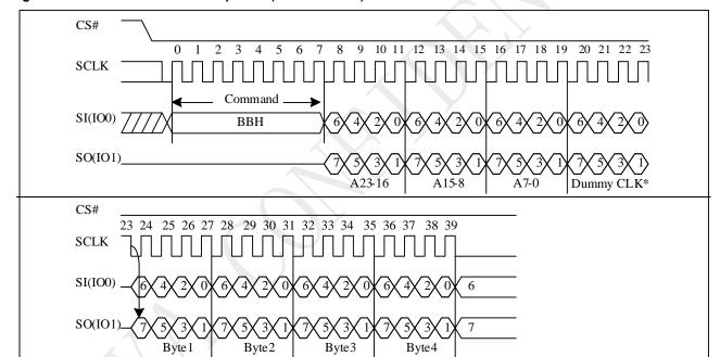
Figure 10-13 2 X IO Read Mode Sequence (Command BB)
