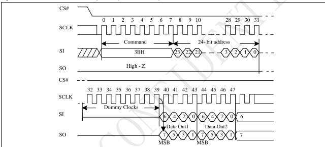
Figure 10-12 Dual Read Mode Sequence (Command 3B)
