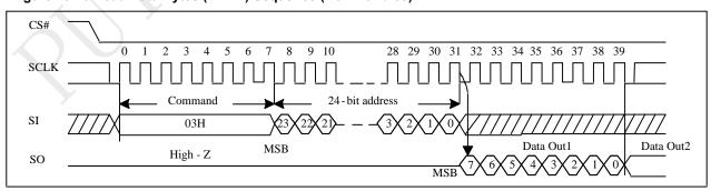
Figure 10-10 Read Data Bytes (READ) Sequence (Command 03)
