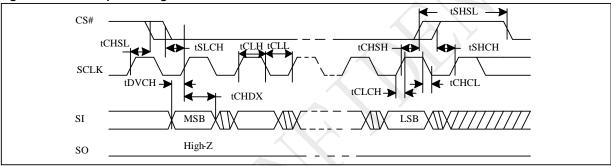
Figure 5-5 Output Timing
