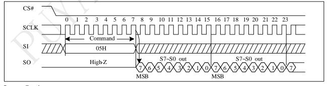
Figure 10-5 Read Status Register (RDSR) Sequence (Command 05)
