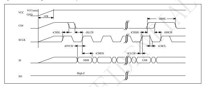
Figure 5-9 Power-up Timing
